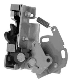
This latch and linkage system is intended for occupant or exit/entry doors for recreational vehicles including motor homes and travel trailers and specialty vehicles including ambulance, fire/rescue and off-highway vehicles (light duty) that require compliance to FMVSS 206 standards. The flexible design allows for internal or external door mounting and provides automotive logic function with remote activating handles.
